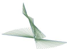
**Figure 33.** The second level interpolated screws with four control screws.
