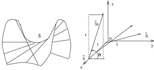
Figure 5. Geometrical illustration of the hyperbolic paraboloid.
