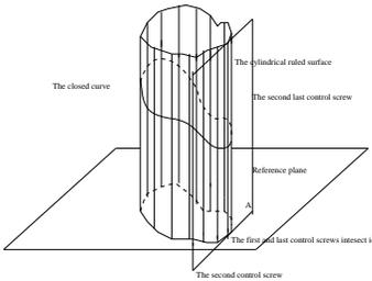
**Figure 12.** The first and last control screws overlap on plane A which is perpendicular to the reference plane
