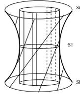
**Figure 24.** The relation between the cylinder and its created hyperboloid.
