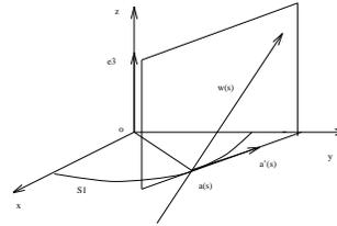
**Figure 25.** The real space geometrical explanation of the ruling of the hyperboloid.
