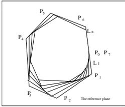
**Figure 10.** When  $t = 0$ , the interpolated line between the first and second control points at any level are identical to the same position interpolated line at the previous level
