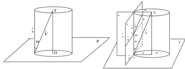
Figure 20. The relationship of rulings of a cylinder and rulings of a cone with a common base curve.
