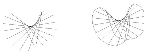
Figure 6. The ruled surface of the hyperbolic paraboloid is drawn by using the dual de Casteljau algorithm.
