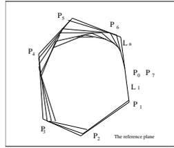
**Figure 11.** When  $t = 1$ , the interpolated line between the last and second to last control points at any level are identical to the same position interpolated line at the previous level
