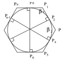
**Figure 15.** Creating a circle with the segment construction method
