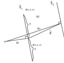
**Figure 30.** Drawing the clipped screw when  $\hat{\mathbf{X}}_1$  is parallel to  $\hat{\mathbf{X}}_2$ .
