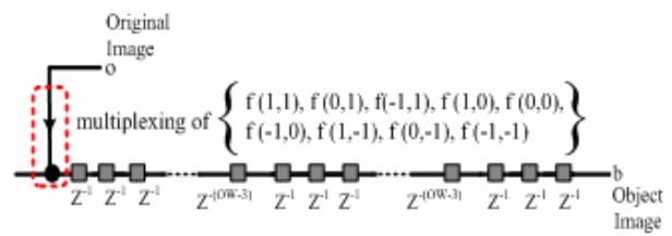
Figure 11. Modified Crookes' implementation with one multiply and one addition delay
