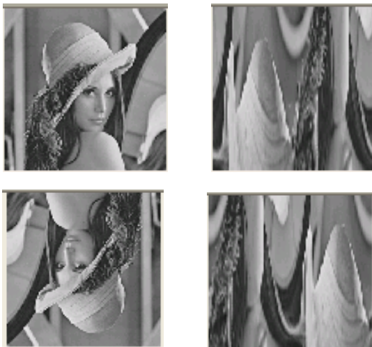
Fig. 2 Log-polar transformation converts the rotation transformation of the original image (from up-left to bottom-left) into a translation transformation (from up-right to bottom-right).
