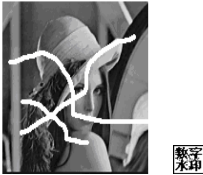
Figure 6. Up-left: watermarked image “Lena” after a cropping distortion and the extracted watermark logo.
