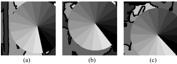
Fig. 10 Results of the sector-wise division for three test images (the watermark-length l is 16): (a) Lena, (b) Baboon, and (c) Peppers. Different sections are filled with different colors.
