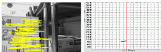
Fig. 16 Left rotated input image, matched feature points with reference image.
