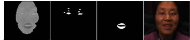
Fig.3. Neural-network based eyes detection. (a) Color-ratio image (b) Upper face segmentation (c) Lower face segmentation (d) Eyes detection
