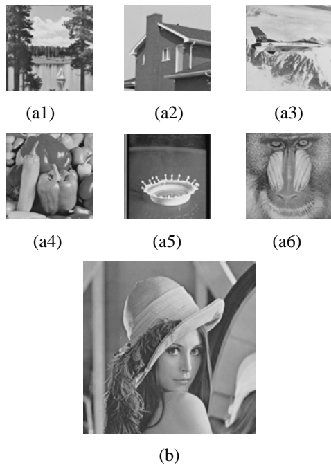
Fig. 3. The output when Lena was first compressed using a ratio of 9. (a) the stego images (PSNRs are all about 52.20dB), and (b) the recovered secret image (whose PSNR was 38.06dB) obtained using “any” four of the six stego images.
