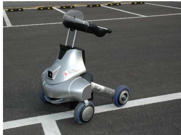
Fig. 9 Implemented walking assistant robot.
