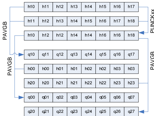
(b) A method to make quarter-pixel for the diagonal element and half-pixel.
