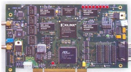
**Figure 5 FPGA BASED Hardware Board**
