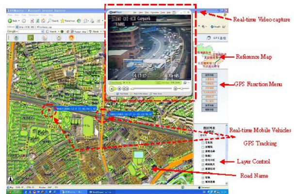
Figure 13. The Screen Copy of Real-time Monitoring of Mobile Vehicles and Video Capture of a Road Cross
