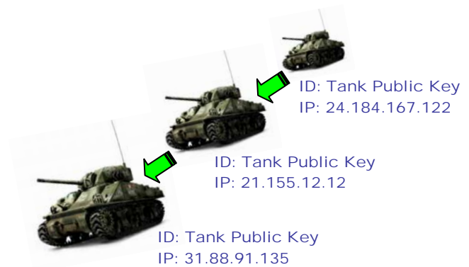
Fig. 11. When moving from one network to another, host id stays same and IP address changes.
