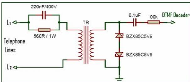
Fig. 6 Magnetic isolation circuit.
