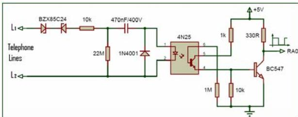
Fig. 5 Optical isolation circuit.
