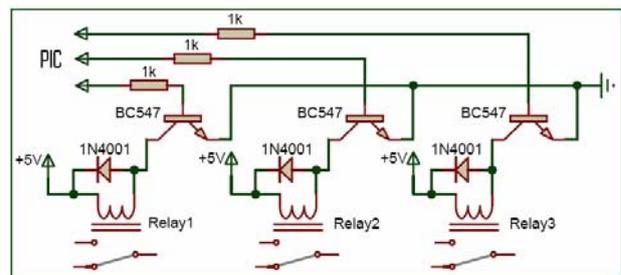
Fig 8 Relay driver circuit
