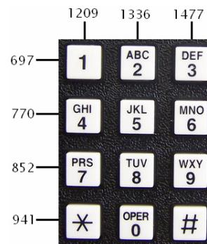
Fig. 2 Keypad with 12 keys and frequencies (Hz).
