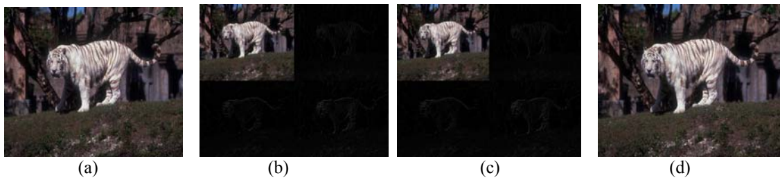
Figure 5(c) : Embedding process (a) Cover Image (b) IWT Image (c) Water Mark Image before IIWT (d) Stegano Image
