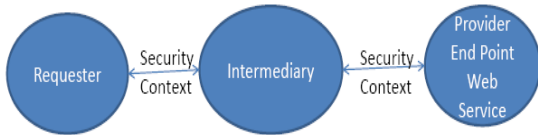
Figure -1.1- Point-to-Point Security establishment
