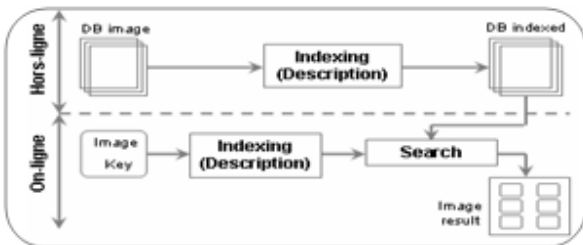
Fig. 4-1: Classic architecture of a CBIR system breaks up into two data processing runs: a “Off-line” phase for indexing or the calculation of the descriptors of the images, and an "On-line" phase of research.
