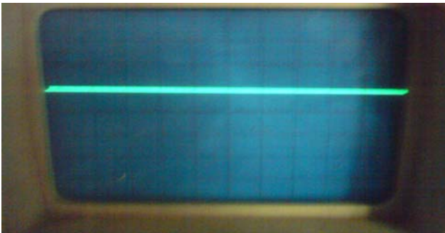
Fig. 21 Oscillogram of output of DC-DC converter
