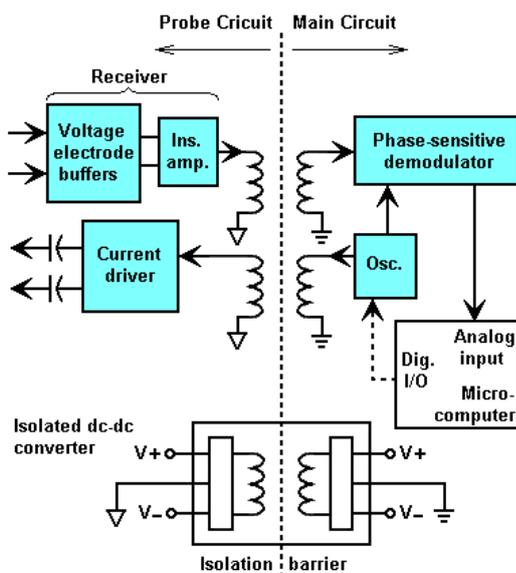
Fig. 1 EIS system architecture
