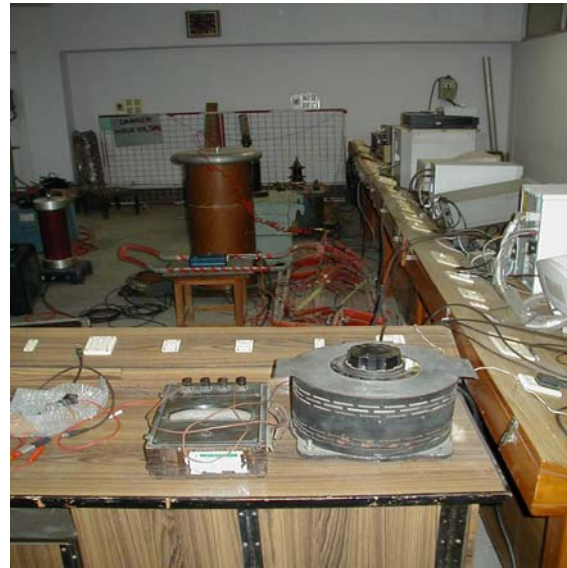
Figure 2.2 PD detection and acquisition setup 2
