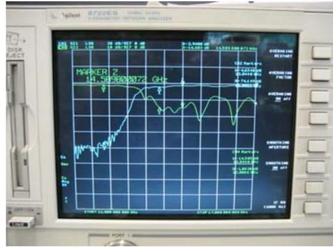
Fig. 9. The test result of the 14GHz HPF, measured by HP 8722ES
