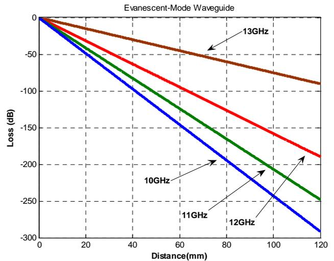
Fig.2. Insertion Loss of SIW with a=7.4mm, h=0.254mm, ε<sub>r</sub>=2.33 and for the length of up to 120mm
