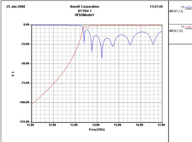
Fig.7.  $S_{11}$  and  $S_{21}$  of the HPF
