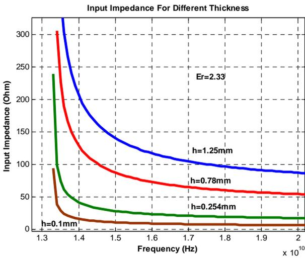
Fig.4. The variation of  $Z_{in}$  by the frequency for different substrate thicknesses and constant  $\epsilon_r$
