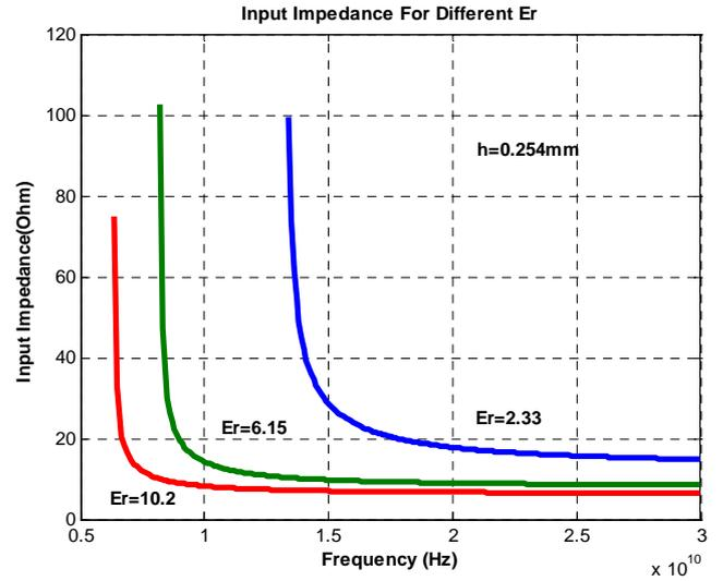
Fig.5. The variation of  $Z_{in}$  by the frequency for different  $\epsilon_r$  and  $h=0.254\text{mm}$
