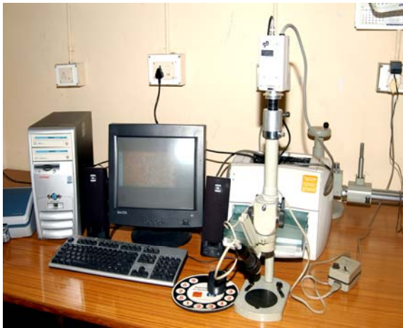
Fig 5 Machine vision system for inspecting surface roughness
