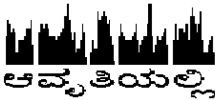
Fig. 8 Character Segmentation by vertical projection profile
