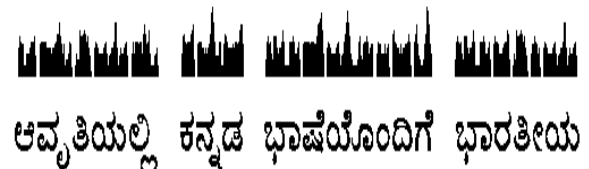
Fig. 7 Word Segmentation by vertical projection profile
