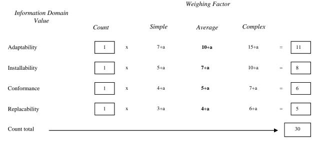
Fig. 7. Computing Function Points for the Portability
