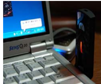
Figure 8. Installing WiBro modem.
