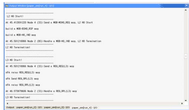
Fig. 4 Handover latency: Application of existing method
