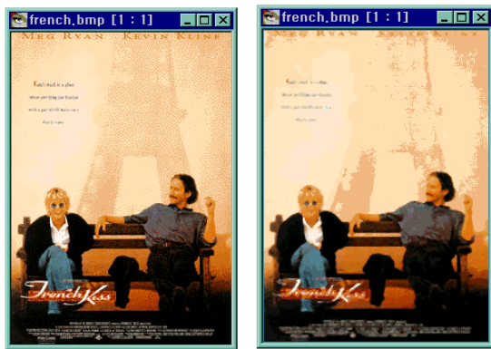
Figure 7 Image modulation using smoothing filter
