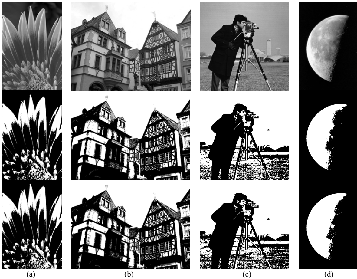
Figure 1. Some samples images from comparison of 5% and 1 % steps. All images from top to bottom: original image, image at 1% step, and image at 5% step. (a) petals.bmp, MSE difference 0.02%. (b) house.bmp, MSE Difference 0.48%. (c) cameraman.bmp, MSE Difference 0.08%. (d) moon.bmp, MSE Difference 4.11%.
