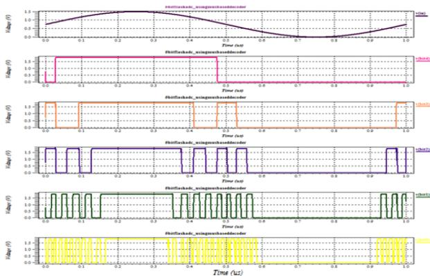
Fig. 7 Transient response of the 5-bit flash ADC for sinusoidal signal of 1MHZ
