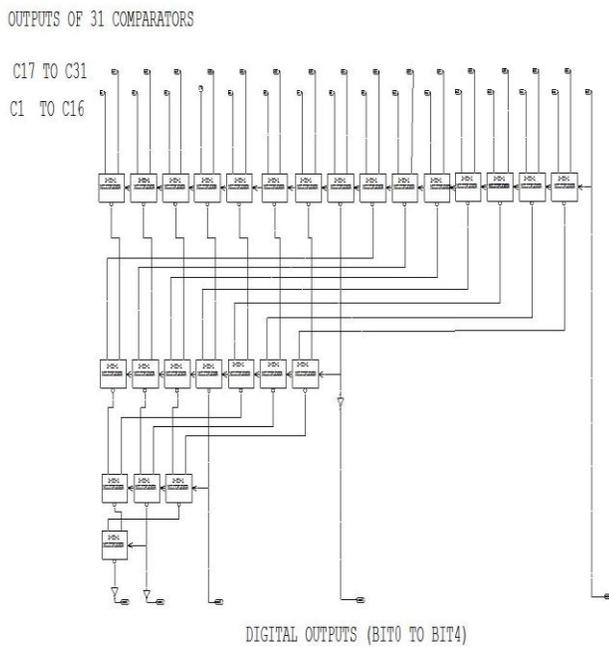
Fig. 4 Multiplexer-based thermometer-to-binary decoder
