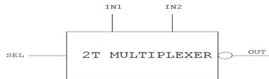
(a) Leaf cell of Multiplexer-based thermometer-to-binary decoder
