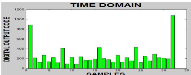
Fig. 10 5-bit flash ADC code coverage
