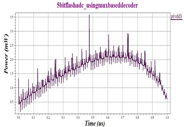
Fig. 9 Instantaneous power plot of the 5-bit flash ADC
