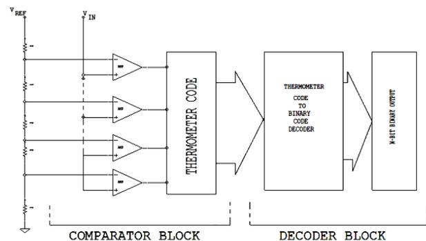
Fig. 1 Architecture of high-speed Flash ADC
