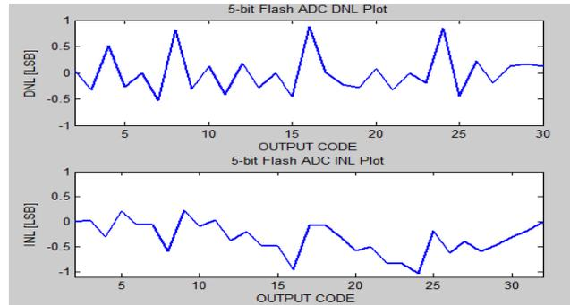
Fig. 11 DNL and INL plot of the designed 5-bit flash ADC
