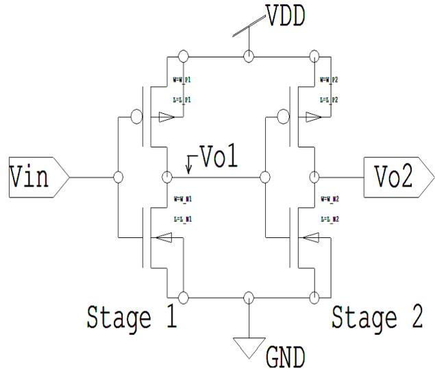
Fig. 3 TIQ comparator schematic
