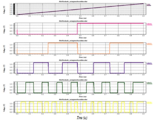
Fig. 8 Transient response of the 5-bit flash ADC for ramp signal
