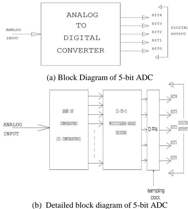
Fig. 2 Schematic representation of 5-bit flash ADC
