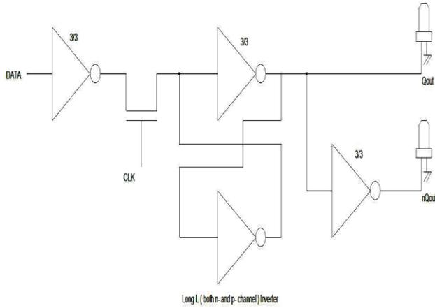
Fig. 6 Inverter based D Flip-Flop implementation
