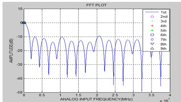
Fig. 12 The FFT plot of the flash ADC
