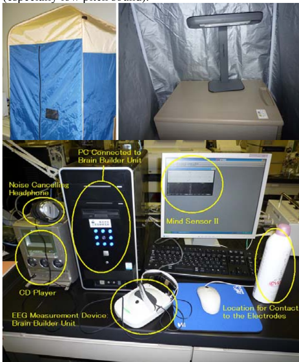
Fig. 6 Experimental equipment for the EEG measurements
