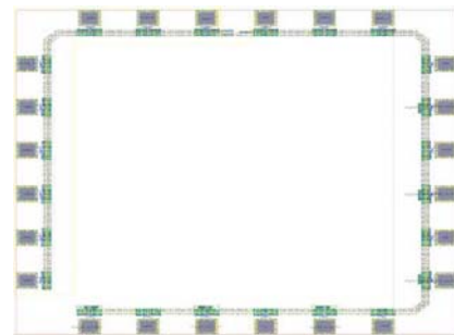
Figure 22 Pad Frame Layout
