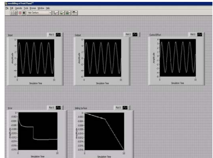
Fig.25. Simulation Results showing Input, Output, Control effort, Error and Sliding surface
