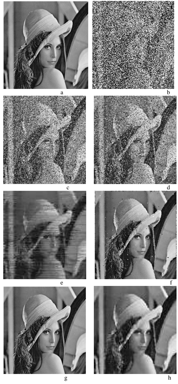
Fig 3. (a) Original Lena image (b) Noisy image of noise density 70%. Restoration results of (c)Standard median filter (d) Weighted median filter (e) Adaptive median filter (f) Decision based algorithm (g) Robust Estimation algorithm (h) proposed method
