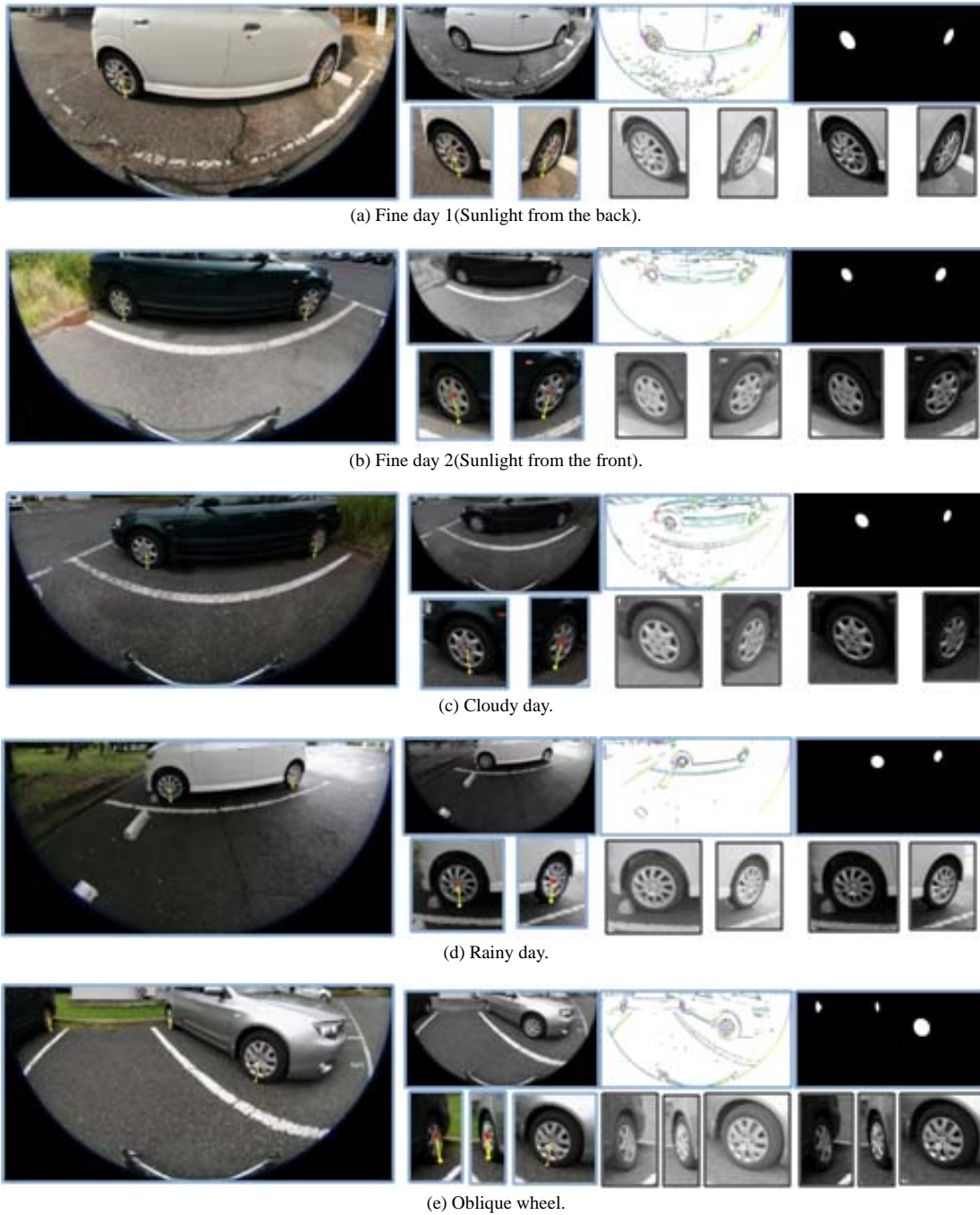
Fig. 9 Results of extraction of wheel regions and detection of tire-road contact points
