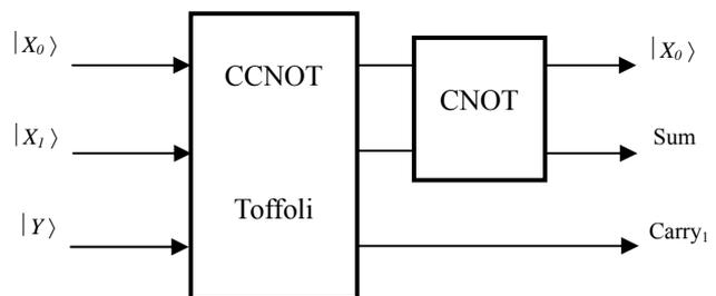
This Circuit represents the three inputs  $(|X_0\rangle, |X_1\rangle, |Y\rangle)$  and three outputs  $(|X_0\rangle, \text{Sum}, \text{Carry}_1)$ .
