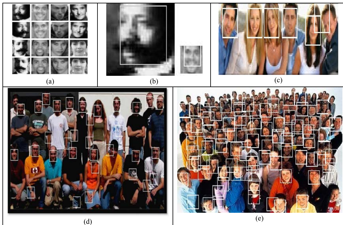
Fig13: (a) Test result on the image created from the training image, (b) Different sized face detection in the same image, (c) Face detection in a simple image, (d) Detection result in a complex image, (e) Result of detection in the exam image
