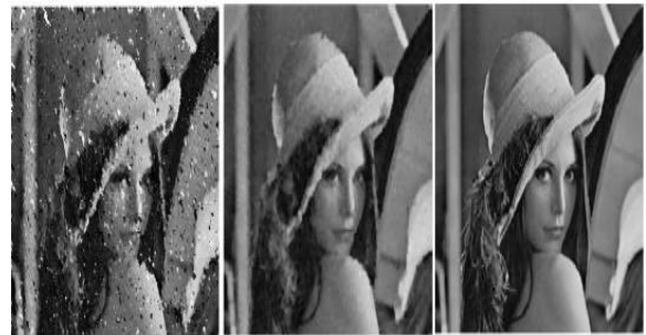
Fig 7.Results of filtering with a 3X3 median and conditional median filter. From left to right, first row: noisy image; second row: Adaptive median filter, Modified Adaptive median filter.
