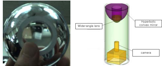
(a) lens part (b) system structure Fig. 5 The structure of the manufactured adaptive omnidirectional vision system.
