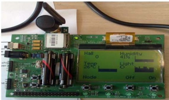
Figure 9 : Jennic active RFID reader (Ref. 29)
