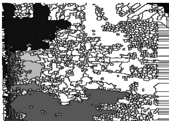
Fig 12. The gradient image of 2-D gel electrophoresis image after applying the Watershed algorithm
