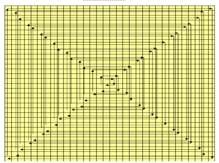
The data read as above format is transposed by writing the data into a new equal sized grid starting from the top left to bottom right column by column. This is as follows.
