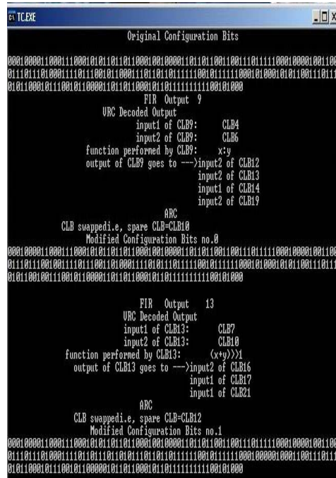
Fig. 11 Autonomously reconfigured VRC for multiple fault CLB scenario
