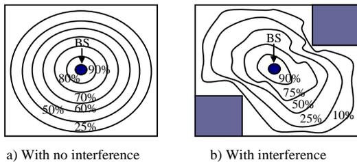
Fig. 3 Signal strength pattern from one BS in a free space
