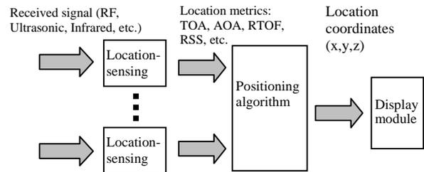
Fig. 1 Functional block diagram of a typical locating system
