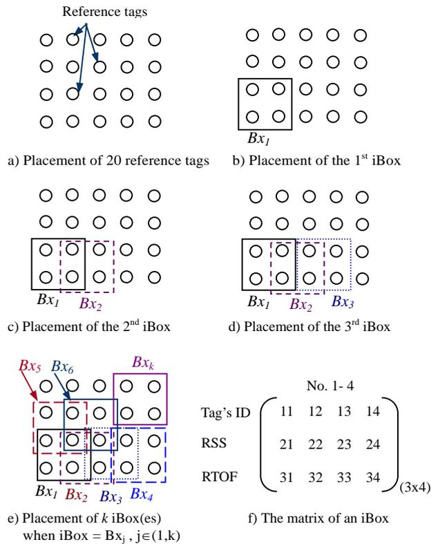
Fig. 4 Placement and generated pattern of the iBox
