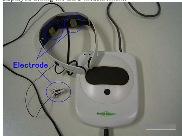
Fig. 2 The Brain Builder Unit with three electrodes
