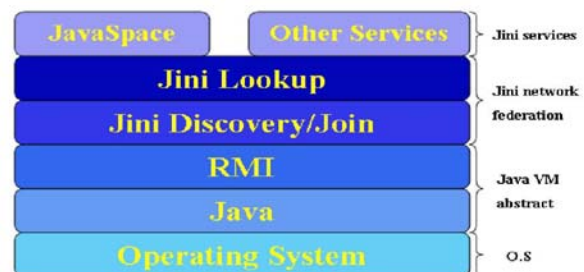
Fig. 1. Jini system architecture
