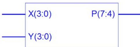
Fig.15: Block diagram of truncated 4x4-bit multiplier
