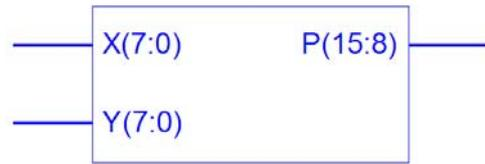
Fig.17: Block diagram of truncated 8x8-bit multiplier
