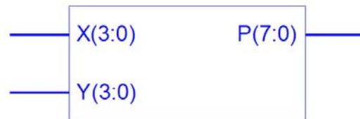
Fig.3: Block diagram of standard 4×4-bit multiplier
