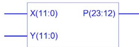
Fig.18: Block diagram of truncated 12x12-bit multiplier
