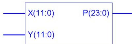
Fig.6: Block diagram of standard 12×12-bit multiplier
