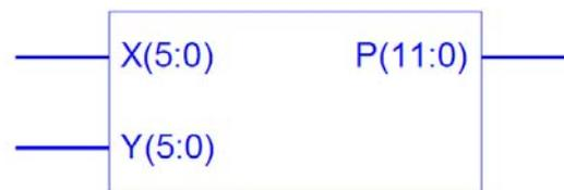
Fig.4: Block diagram of standard 6×6-bit multiplier
