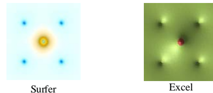
Fig. 8. Reservoir pressure distribution. Filled-up image
