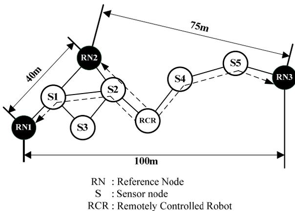
Fig. 2.1 DV-HOP algorithm for recognizing locations of the remotely controlled robot
