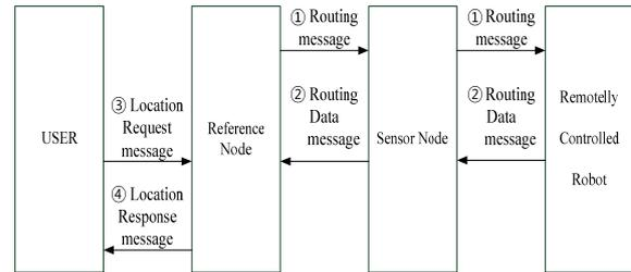
Fig. 3.6 Message Flow diagram of the location recognition in the RDV-HOP algorithm
