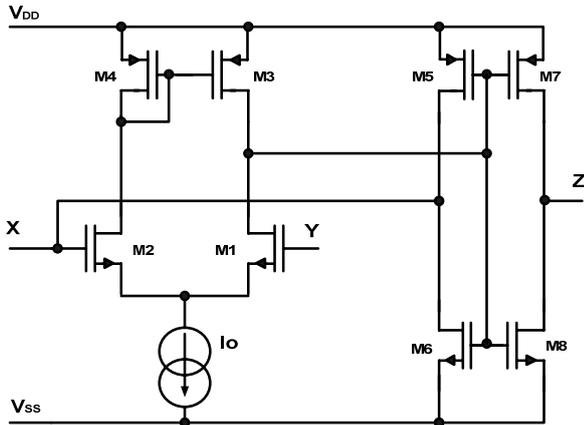
Fig. 8 A differential pair Class AB current conveyor.
