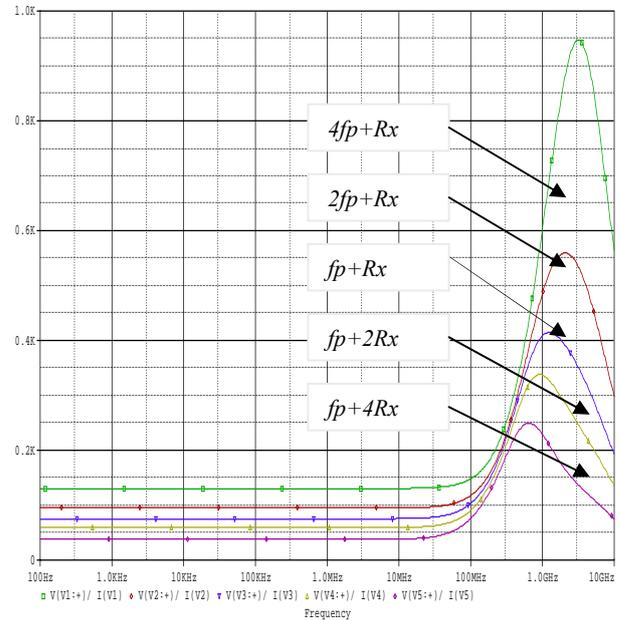
Fig. 13 Rx ( $\Omega$ ) vs. frequency (Hz), for different values of  $\gamma_i$ .
