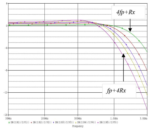
Fig. 14 Current gain (dB) vs. frequency (Hz), for different values of  $\gamma_i$ .
