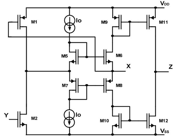
Fig. 12 The inverted second-generation CMOS current conveyor.
