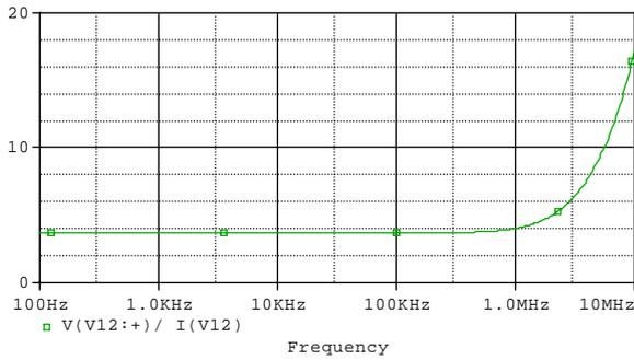
Fig. 10 Rx-pole resistance (Ω) vs. frequency (Hz),
