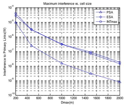
FIGURE 6: HIGHEST INTERFERENCE VS. CELL SIZE
