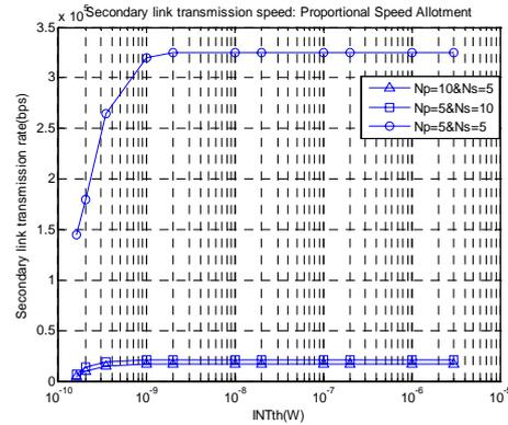
FIGURE 3: SECONDARY LINK TRANSMISSION RATE: PSA
